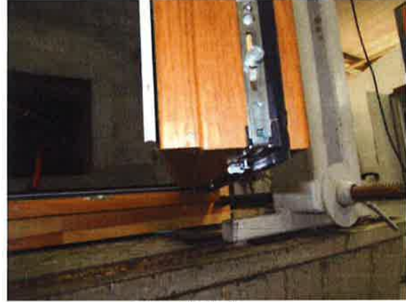
Picture 2 Internal rebate seal
