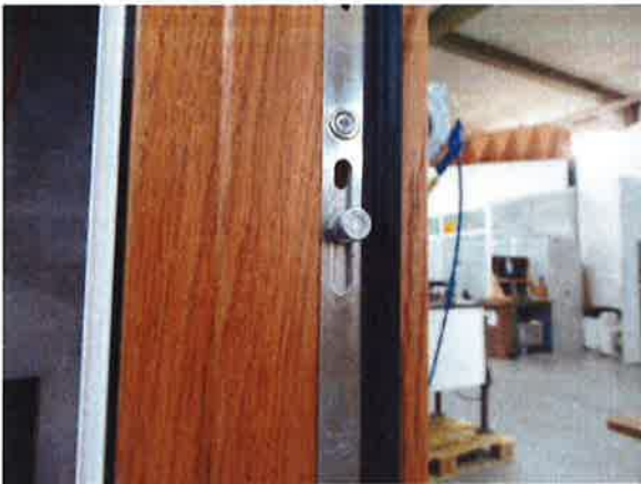
Picture 15 Locking situation frame member 4
